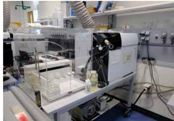
Inductively coupled plasma mass spectrometry (ICP-MS) for simultaneous ultratrace analysis of metals and single-particle nanomaterial analysis.
