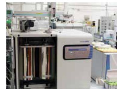
The elemental analyser-isotope ratio mass spectrometer represents the workhorse for carbon and nitrogen stable isotope analyses in bulk materials, such as in soils, plants and microbes.
