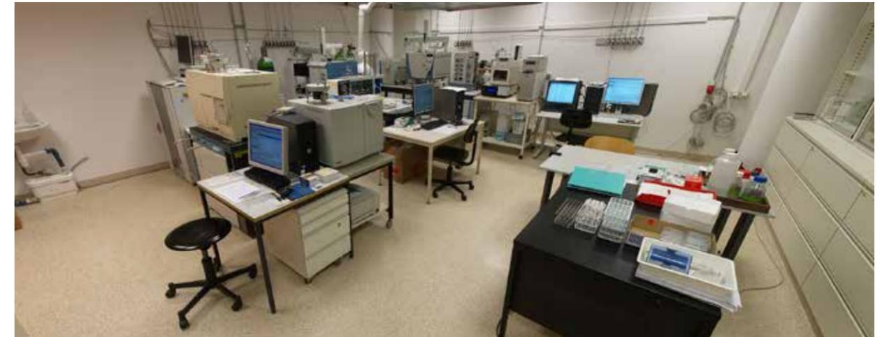
Overview of SILVER laboratory with five isotope ratio mass spectrometers allowing bulk and compound-specific analysis of hydrogen, carbon, nitrogen and oxygen in biological and environmental samples.
