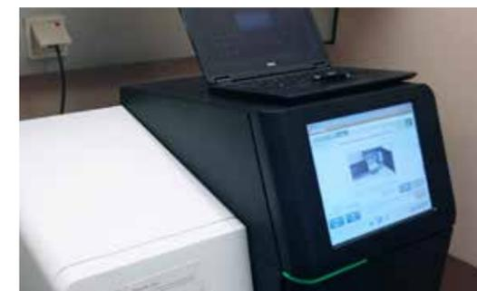
The Illumina MiSeq System, our high quality short read sequencing technology of choice, is applied for data generation in the JMFs amplicon sequencing pipeline.
