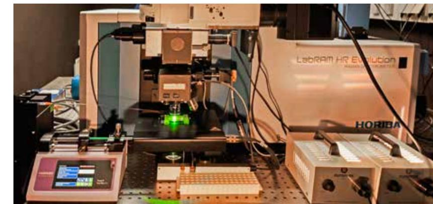
**A Raman microspectrometer that is used for analysing the chemical and isotope composition of single microbial cells, and for sorting single cells based on their in situ metabolic activities in environmental and medical samples.**
