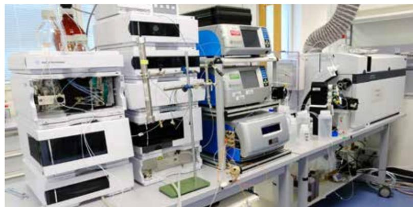
**Field Flow Fractionation nanoparticle separation system coupled to various detection systems for detailed characterisation (UV-DAD, Fluorescence, DRI, static & dynamic light scattering and ICP-MS/MS).**
