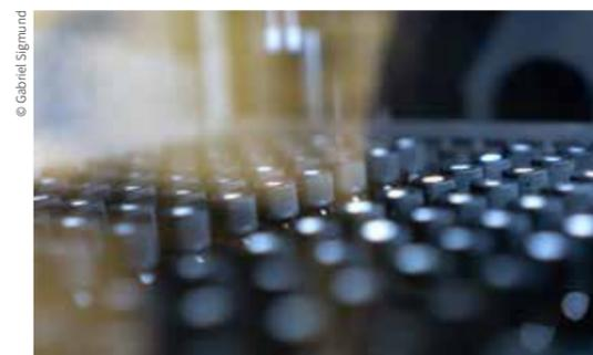
**Soil extracts containing organic contaminants on an auto sampler for analysis via liquid chromatography-mass spectrometry (LC-MS/MS).**
