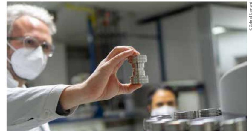
**Accelerated Solvent Extraction – Organic pollutants are extracted from solid samples as soil or sediments at high temperature and pressure.**
